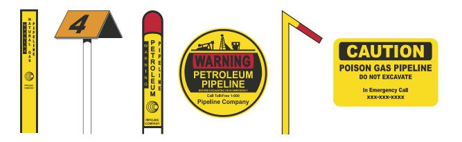
Markers warn that a transmission pipeline is located in the area, identify the product transported in the line, and provide the name and telephone number of the pipeline operator to call. Markers and warning signs are located at frequent intervals along natural gas and liquid transmission pipeline rights-of-way, and are located at prominent points such as where pipelines intersect streets, highways, railways, or waterways.
